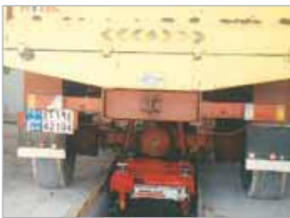
P300 hand pump and 10 ton cylinders used for a vehicle lift.
