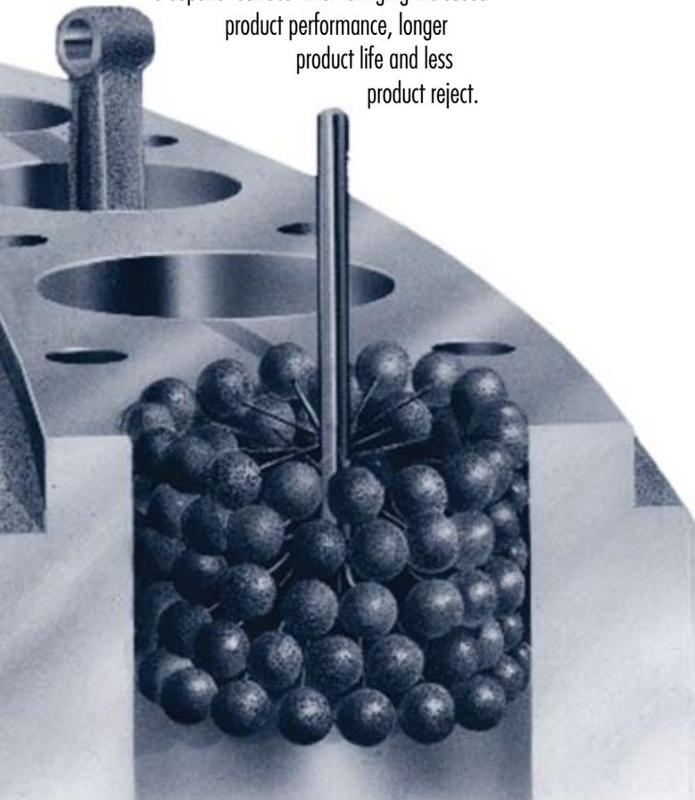
Each abrasive globule is attached to high density nylon filament to enhance durability
